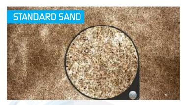
Dry siliceous natural sand calibrated to 0/2mm conforming to norm EN 196-1 and ISO 679: 2009. Used to control the mechanical resistance of cements and other hydraulic binder.
